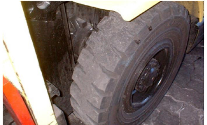
**Yard machine.** This machine works 100% of the time on surface shown in this photo. This machine loads and off loads pallets. This machine has worked for on 4240.7 Hrs on the set of tyres shown. Before fitting the TXP this machine was achieving +/- 1800hrs per set of front tyres. These tyres were replaced at over 5000hrs.
